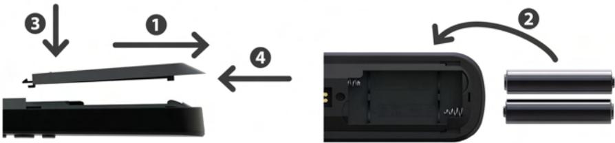
**Figure 2:** Inserting the batteries
